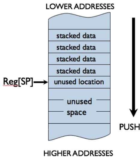
**PUSH(X)**: Push  $\text{Reg}[x]$  onto stack
