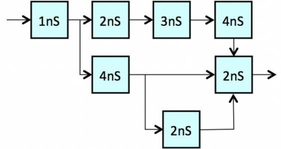
(C) (2 points). Show the maximum-throughput 3-stage pipeline using a minimal number of registers.
