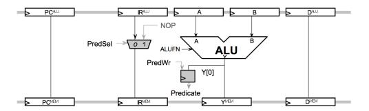
Comparison instructions write the 1-bit predicate register (the PredWr control signal ensures that only comparison instructions update the register). The PredSel mux annuls ALU instructions if they are predicated and should not execute according to the value of the predicate register.
