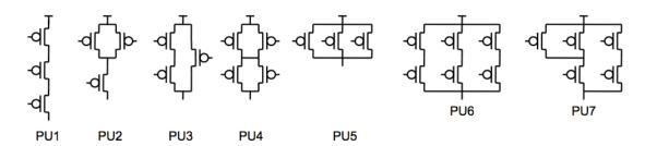
The web site explains that the customer can choose which inputs are connected to each PFET, allowing their pullups to be used in various ways to build gates with various numbers of inputs. Since Pullups Galore charges by transistor, you are interested in selecting pullups using the minimum number of transistors for each of the 3-input gates you are designing.
