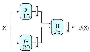
Now F & G can be working on input  $X_{i+1}$  while H is performing its computation on  $X_i$ . We've created a 2-stage *pipeline*: if we have a valid input X during clock cycle j, P(X) is valid during clock j+2.
