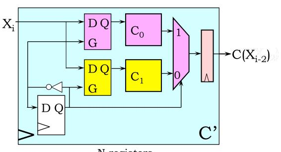
N-way interleaving is equivalent to N pipeline Stages...
