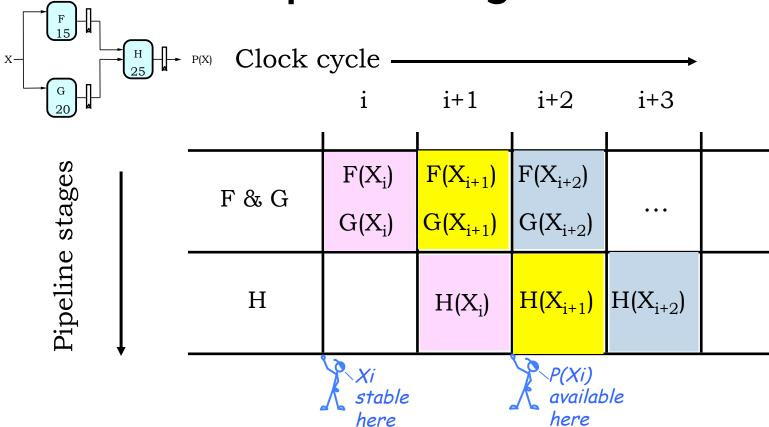
The results associated with a particular set of input data moves *diagonally* through the diagram, progressing through one pipeline stage each clock cycle.
