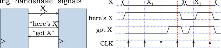
Asynchronous, locally-timed system using transition signaling:
