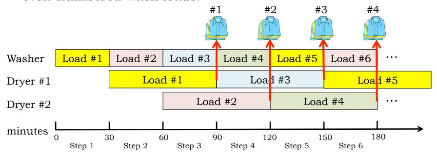
Throughput =  $\frac{1/30}{100}$  loads/min, Latency =  $\frac{90}{1000}$  mins/load
